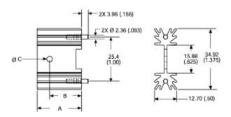
A Dim **38.1 (1.50)** B Dim **18.29 (.720)** C Dim **3.18 (.125)**
